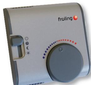
By using the Froling **room temperature sensor FRA** the most important modes of the heating circuits can be adjusted. The adjusting wheel allows you to change the room temperature by up to +/- 3° C.
